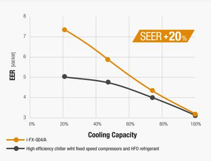
The increase in efficiency compared to high efficiency ErP 2018 compliant fixed speed units is expressed by drawing the EER trend to the conditions defined by the ErP directive 2009/125 /EC necessary for the calculation of SEER seasonal parameters.
